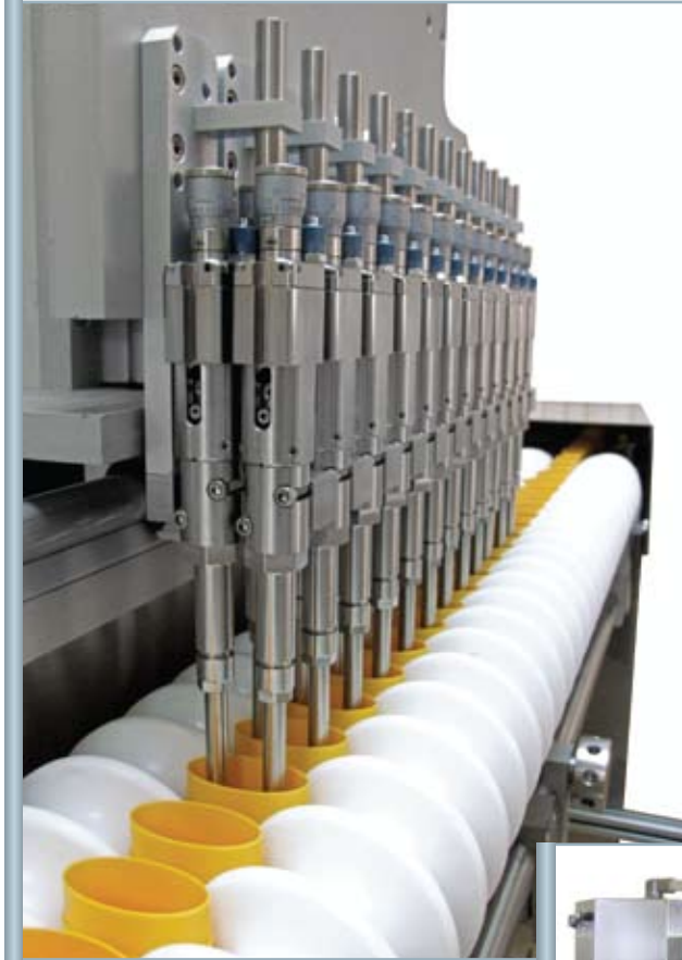
Provision for Servo Motor Controlled Bottom/Up Fill Motion for high viscosity products or foamy products.
